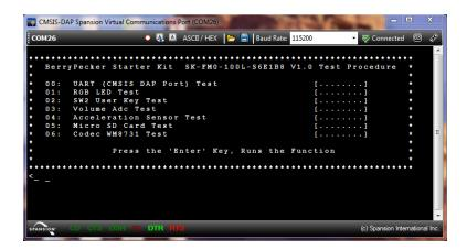
5) To run each of the tests, enter the number next to the test description and follow the prompts. For example: Input 4 and press Enter will run the Acceleration Sensor Test. The application will output the value of the sensor and loop until the Enter key on the PC keyboard is pressed.
